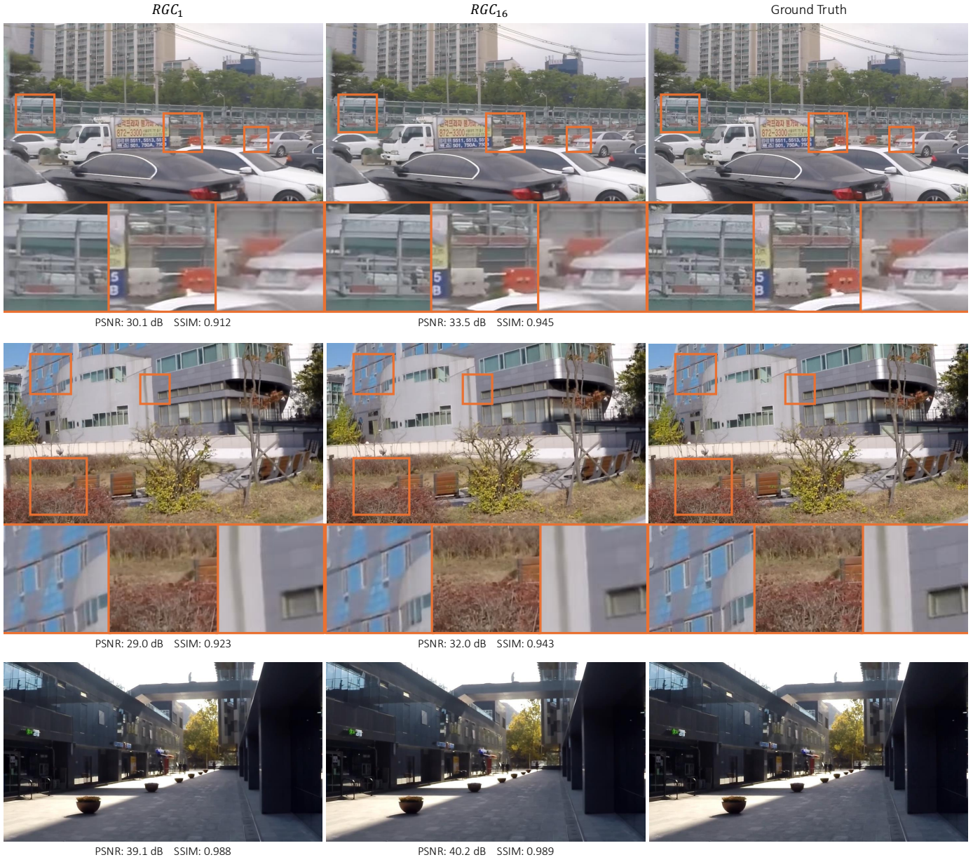
Fig. S6. Interpolation reconstructions from RGC_1 and RGC_{16} : We show the middle reconstructed frame for the one learned kernel and 16 learned kernel models trained at the ultra-low bandwidth of roughly 10,000 events.
