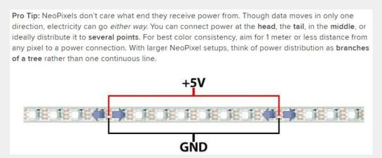
Supply separate 5V to the pixels instead of having the arduino power it. The Arduino can only continuously supply about 500mA to the 5V pin. Each Neopixel can draw up to 60 mA at full brightness.
